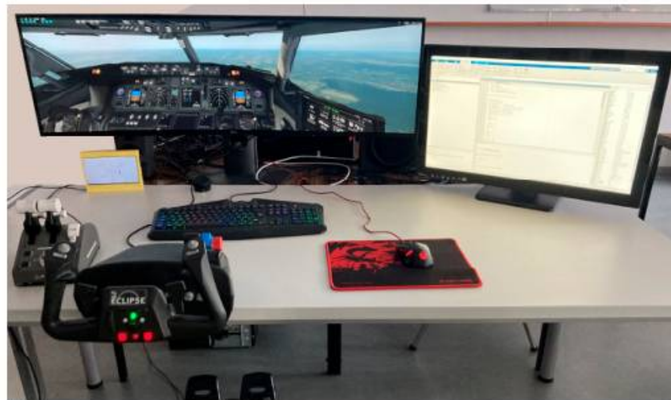
Figure 7. Stationary simulator stand with cockpit view of a jet airliner—Boeing 737-800.
